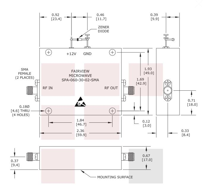
HEAT SINK REQUIRED FOR PROPER OPERATION, UNIT IS COOLED BY CONDUCTING TO HEAT SINK.
