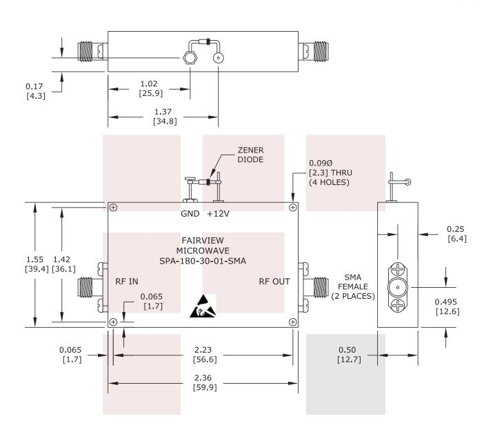
HEAT SINK REQUIRED FOR PROPER OPERATION, UNIT IS COOLED BY CONDUCTING TO HEAT SINK.
