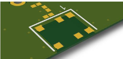
The clear-out area is simply defined as the same size as the antenna. No additional clearance is required.
