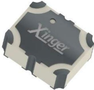
The X4C30K1-20S is a low profile, high performance 20 dB directional coupler in a new easy to use, manufacturing friendly surface mount package. It is designed particularly for LTE and 5G wireless communication frequency bands. The X4C30K1-20S is designed particularly for power and frequency detection, as well as for VSWR monitoring, where tightly controlled coupling and low insertion loss is required.
