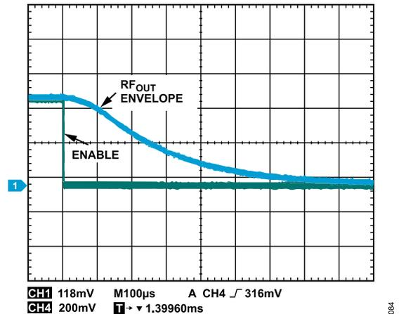
Figure 82. Turn-Off Response Time of the RF<sub>OUT</sub> Envelope When IN Pin of the ADG719 Is Pulsed
