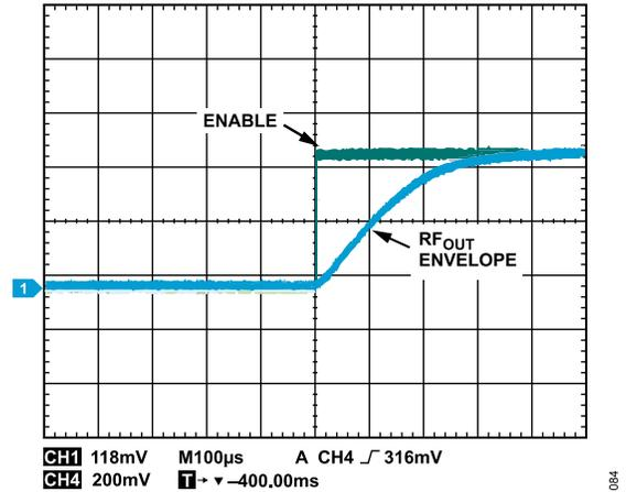
Figure 81. Turn-On Response Time of the RF Output (RF<sub>OUT</sub>) Envelope When IN Pin of the ADG719 Is Pulsed
