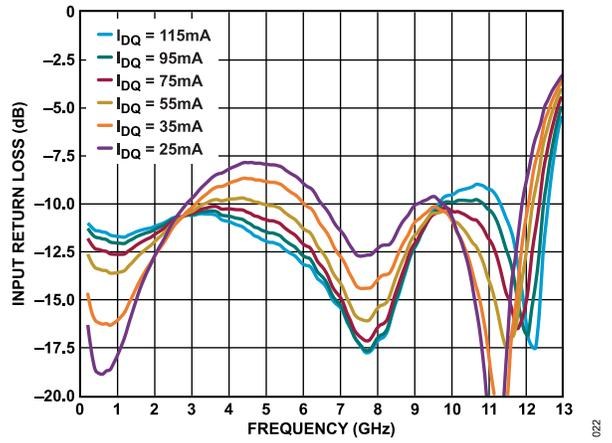
Figure 22. Input Return Loss vs. Frequency for Various  $I_{DQ}$  Values, 200 MHz to 13 GHz,  $V_{DD} = 5\text{ V}$
