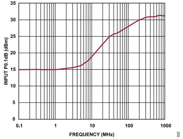
Figure 22. Input P0.1dB vs. Frequency, Low Frequency Detail
