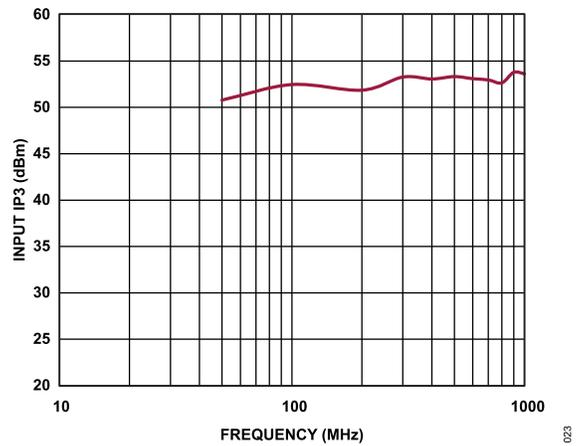
Figure 23. Input IP3 vs. Frequency, Low Frequency Detail
