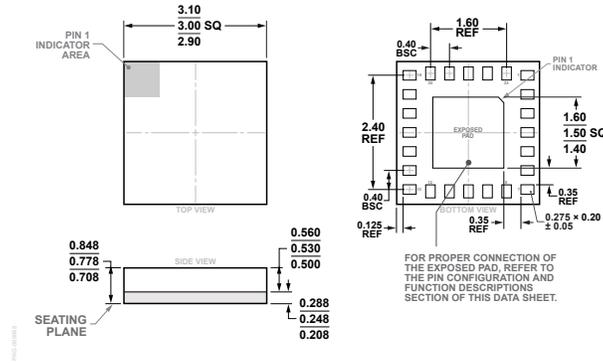
Figure 28. 24-Terminal Land Grid Array [LGA]
