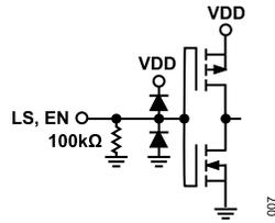
Figure 7. LS and EN Control Interface Schematic
