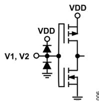
Figure 6. V1 and V2 Control Interface Schematic
