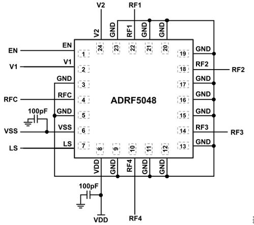
Figure 24. Recommended Schematic
