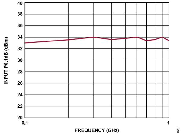
Figure 25. Input P0.1dB vs. Frequency, Low Frequency Detail
