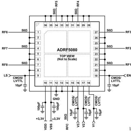
Figure 27. Recommended Schematic
