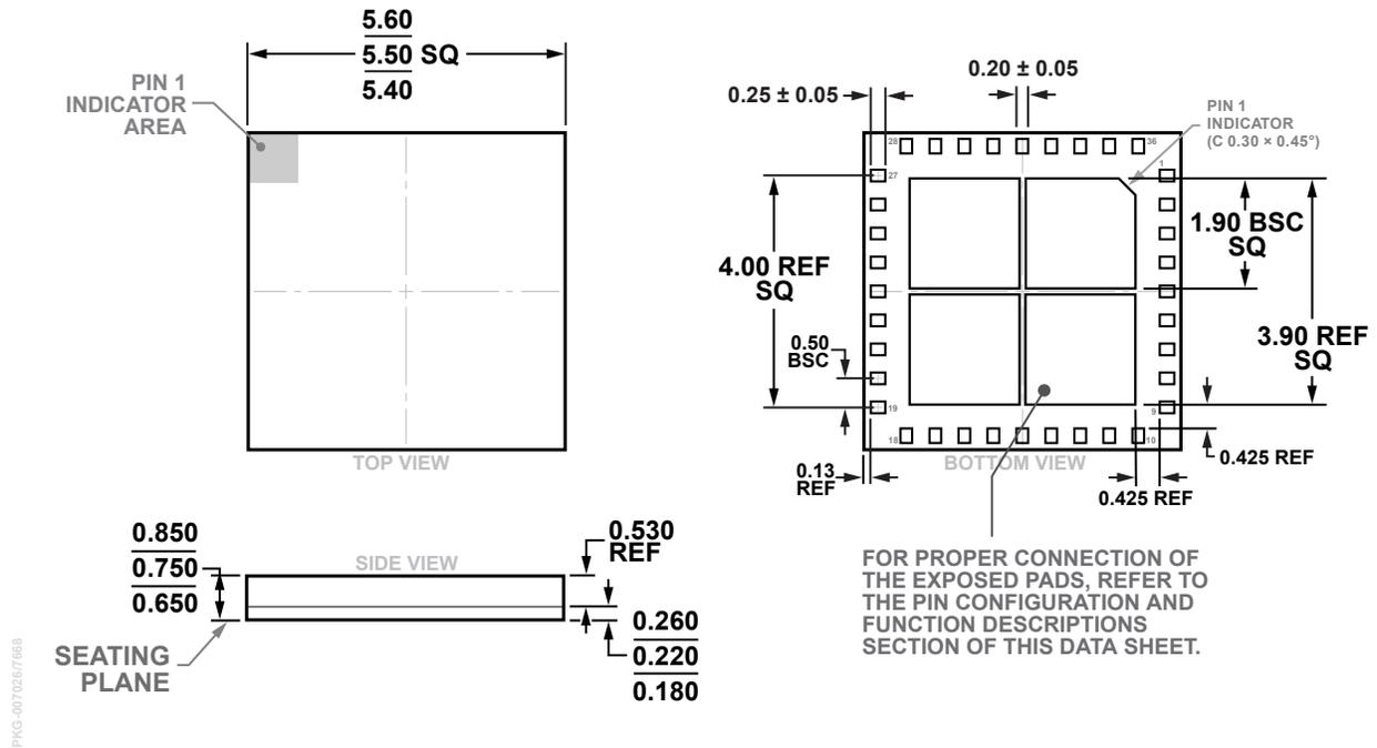
Figure 31. 36-Terminal Land Grid Array [LGA] (CC-36-2)
