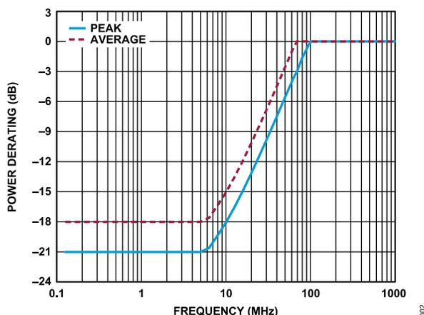
**Figure 2. Power Derating vs. Frequency, Low Frequency Detail, T<sub>CASE</sub> = 85°C**
