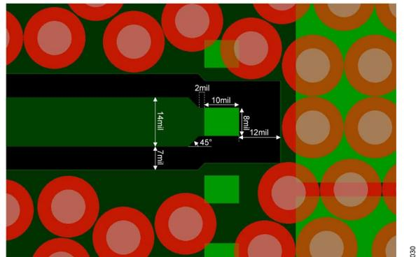
Figure 30. Recommended RFx Pin Transitions
