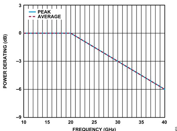
**Figure 3. Power Derating vs. Frequency, High Frequency Detail, T<sub>CASE</sub> = 85°C**
