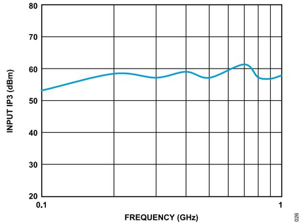
Figure 26. Input IP3 vs. Frequency, Low Frequency Detail
