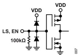
Figure 7. LS and EN Interface Schematic
