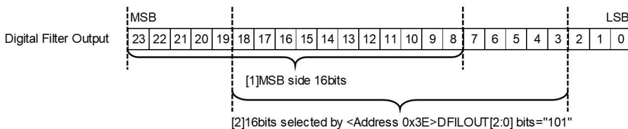
Figure 60 Digital Filter Output bit Structure (eg. DFIOUT bits= "101")
