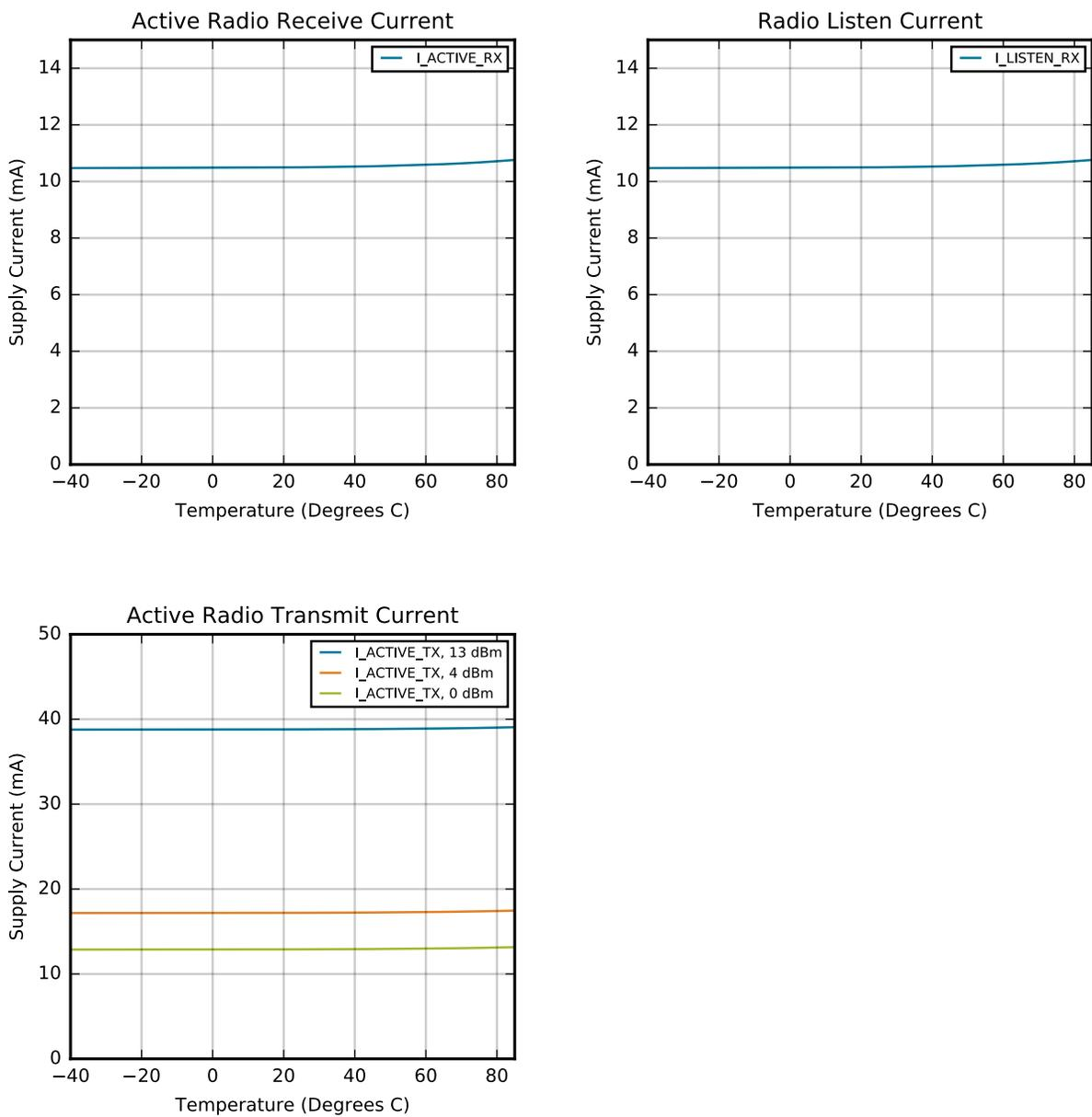
Figure 4.2. Supply Current vs. Temperature
