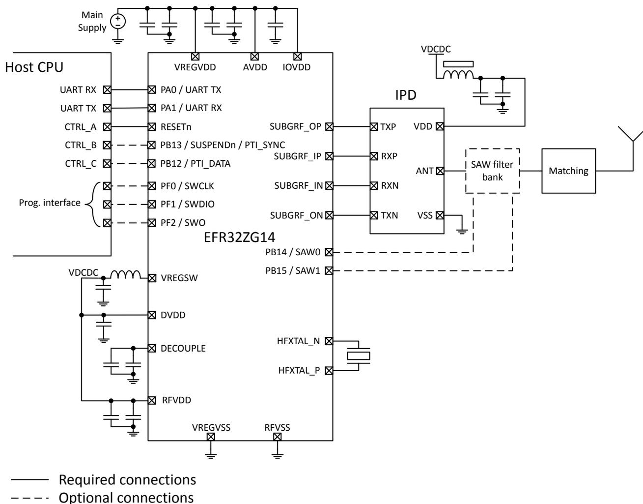
Figure 5.1. Typical System Connections for Z-Wave with IPD
