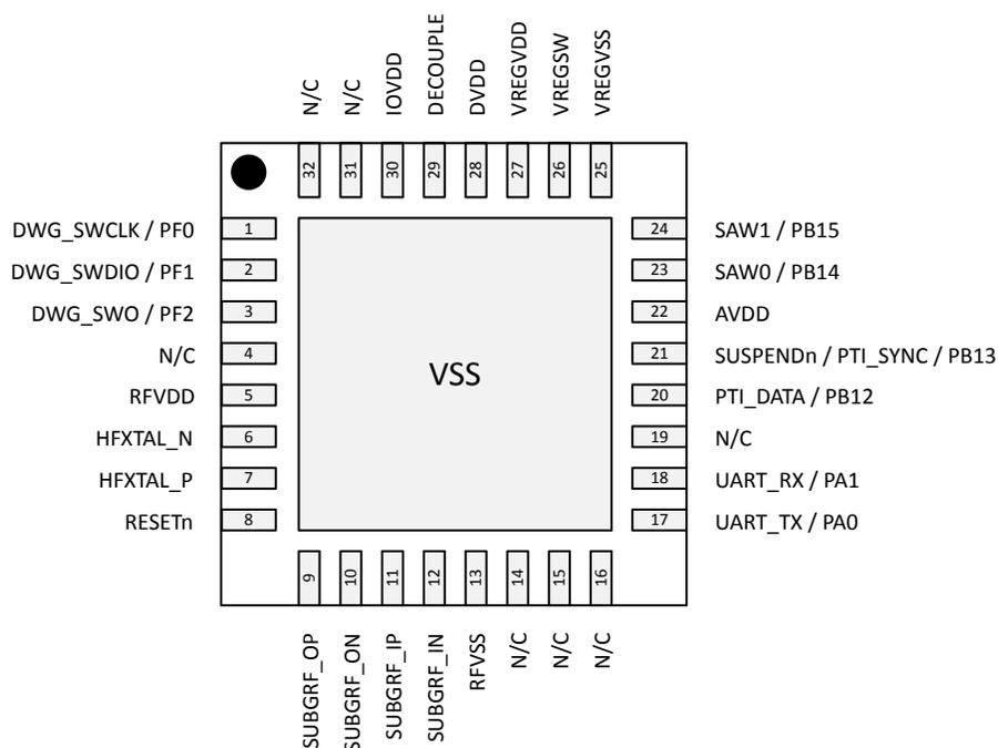
Figure 6.1. EFR32ZG14 Device Pinout
