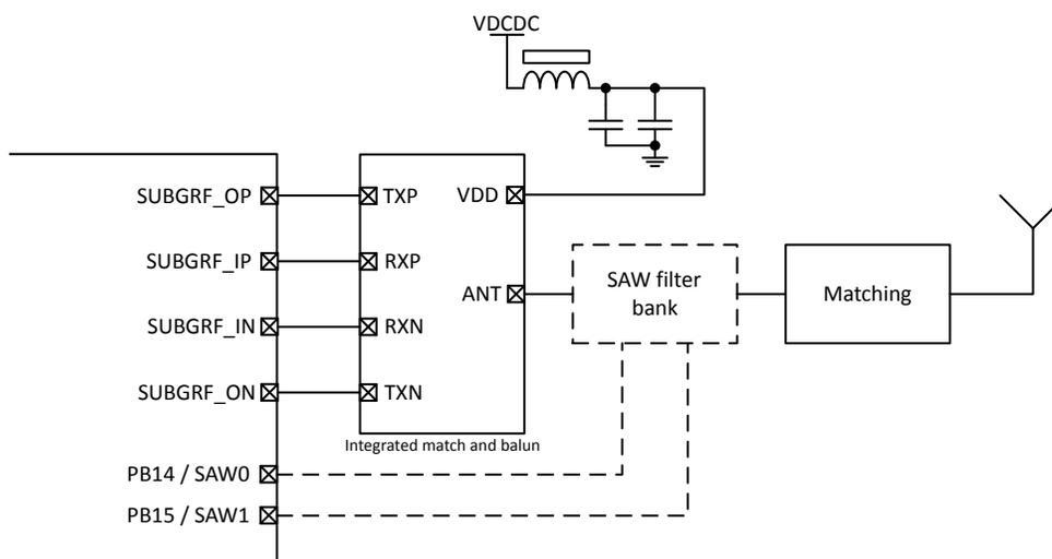
**Figure 3.2. Radio Interface with IPD**
