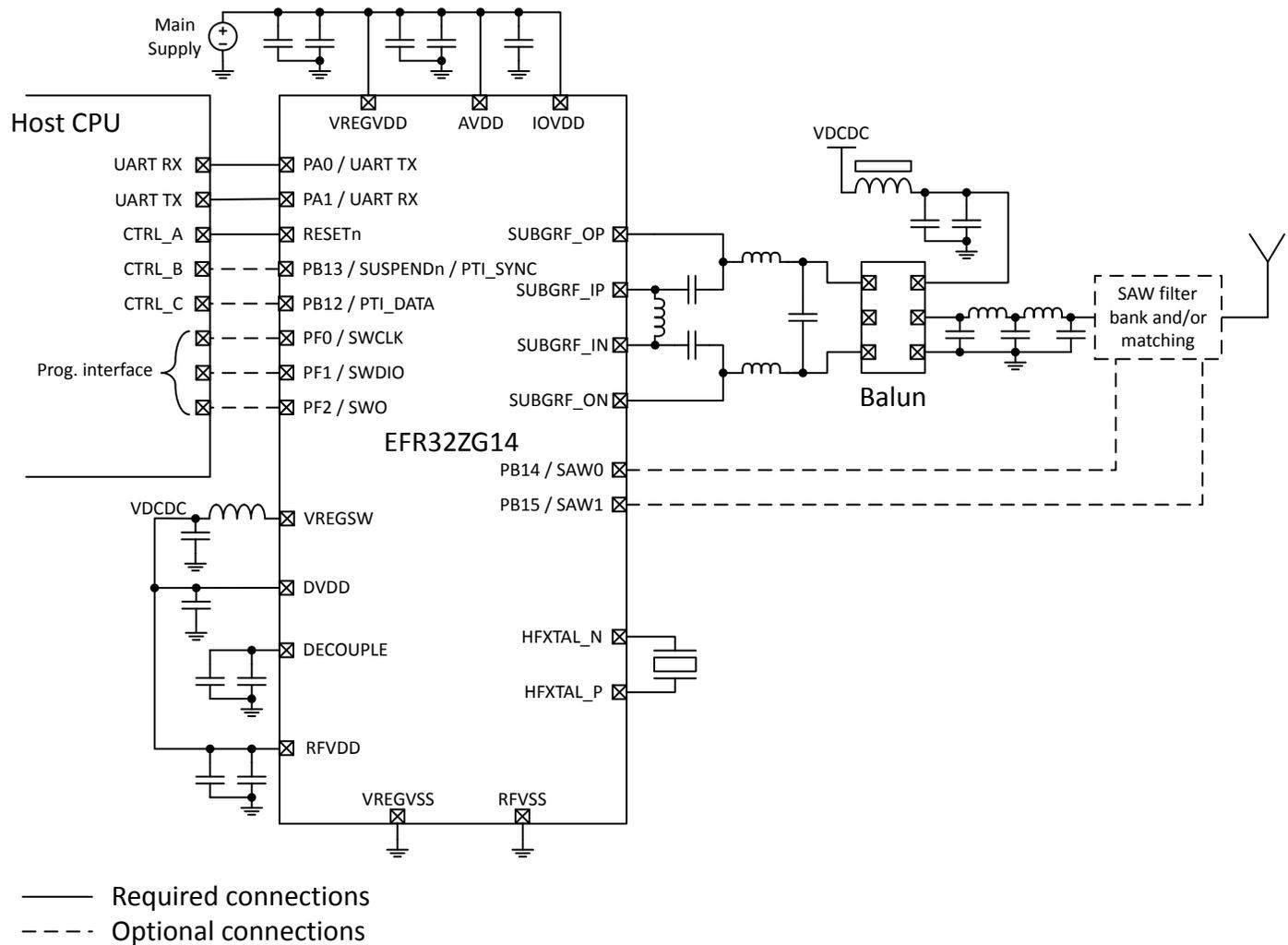
Figure 5.2. Typical System Connections for Z-Wave Long Range
