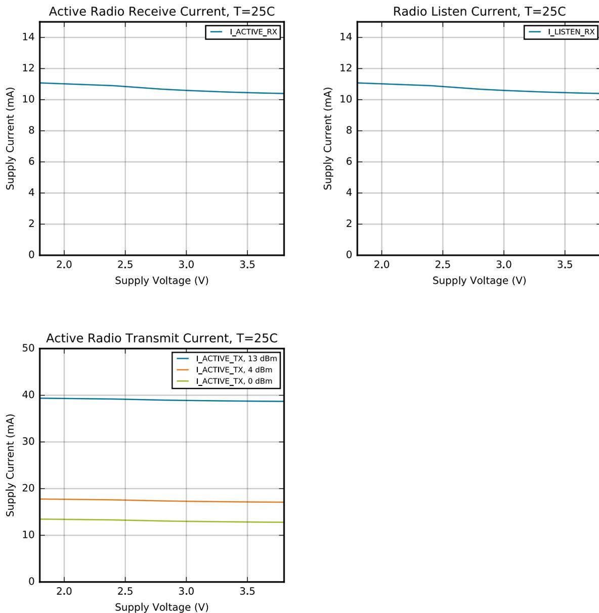
Figure 4.1. Supply Current vs. Supply Voltage
