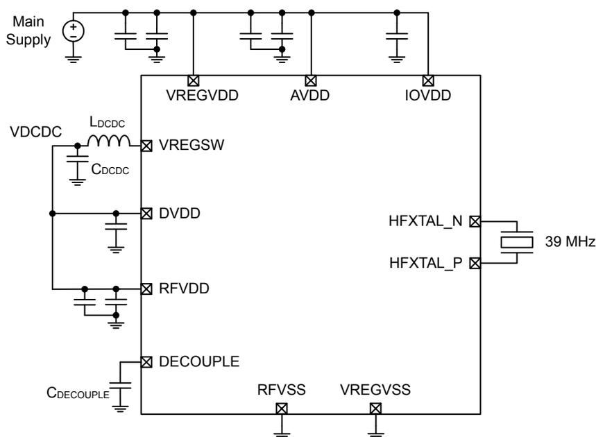
Figure 3.1. Power Supply Connections
