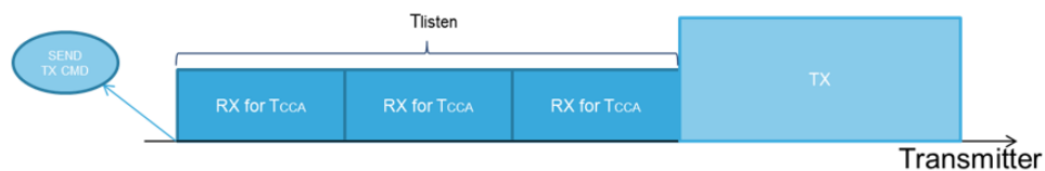
Figure 23. CSMA if channel is free (timeline)
