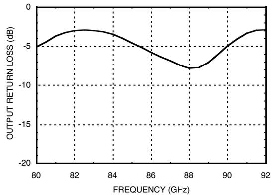
Note: Measured Performance Characteristics (Typical Performance at 25°C) Vdd1 = Vdd2 = 4V, Idd1 = 80mA, Idd2 = 80mA
