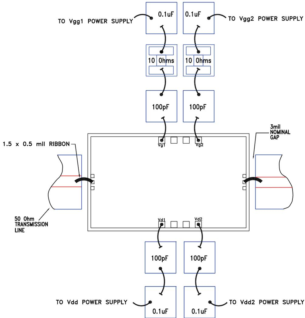
Note 1: Bypass caps should be 100 pF (approximately) single-layer placed no farther than 30 mils from the amplifier.
