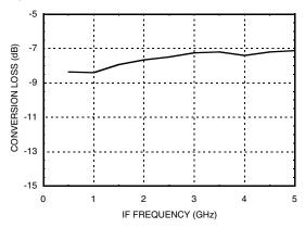
Note: Measured Performance Characteristics (T<sub>OP</sub> = 25°C)
