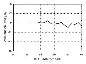
Note: Measured Performance Characteristics (T<sub>OP</sub> = 25°C)
