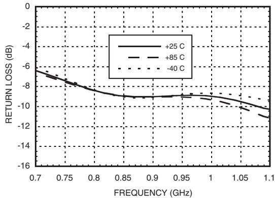
**Output Return Loss vs. Temperature @ 900 MHz**
