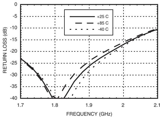
**Output Return Loss vs. Temperature @ 1900 MHz**
