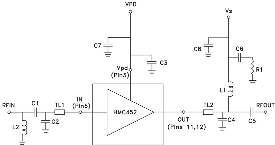
Note: C2, C3 and C4 should be placed as close to pins as possible.
