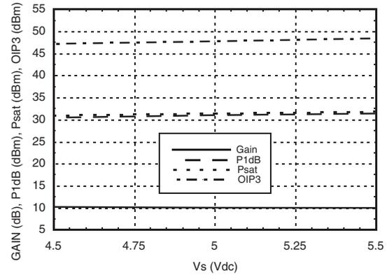
**Gain, Power & IP3 vs. Supply Current @ 1900 MHz\***
