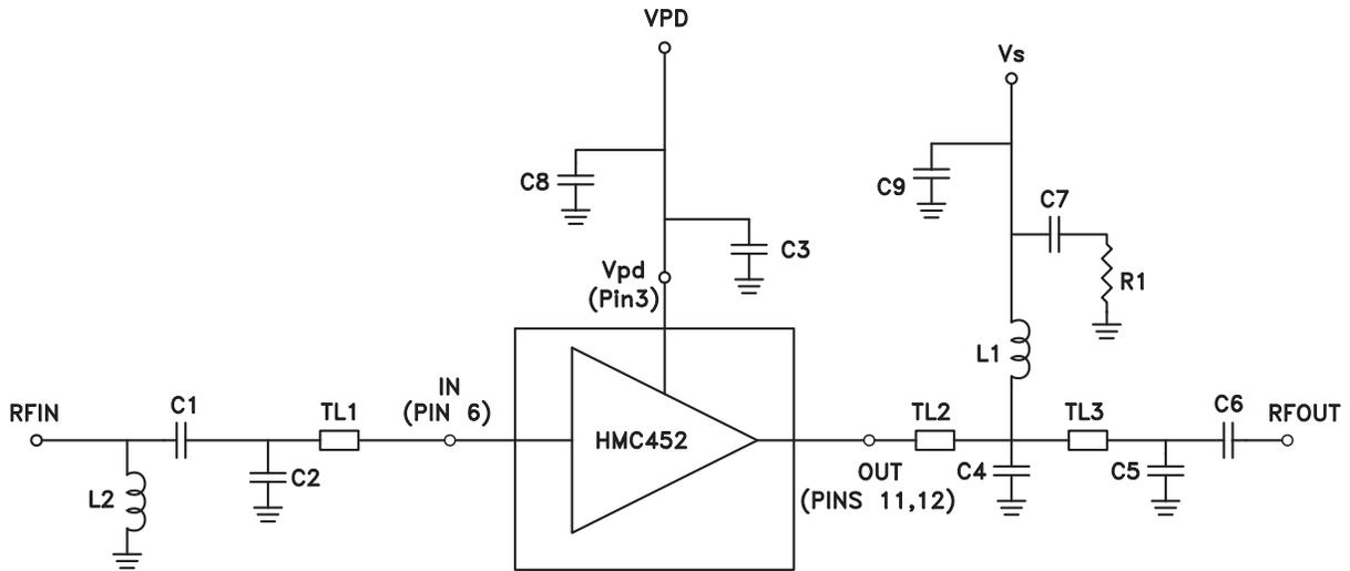
Note: C3 should be placed as close to pins as possible.
