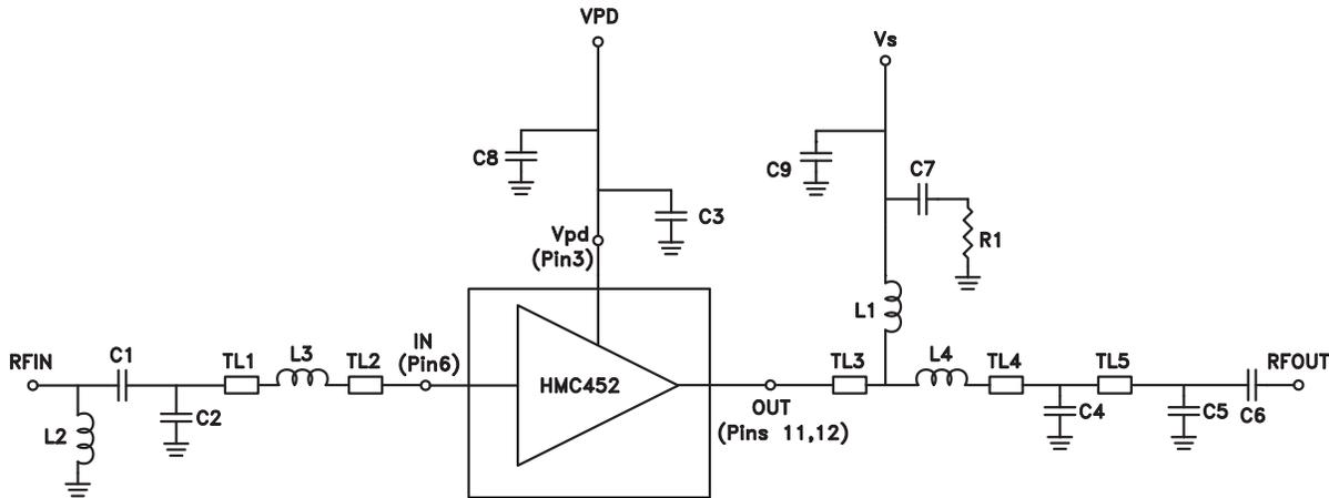
Note: C3 should be placed as close to pins as possible.
