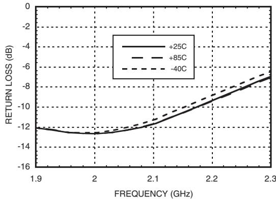
**Output Return Loss vs. Temperature @ 2100 MHz**
