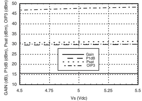
**Gain, Power & IP3 vs. Supply Current @ 900 MHz\***
