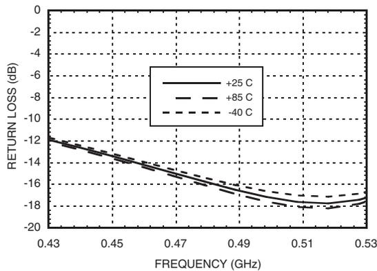
**Output Return Loss vs. Temperature @ 470 MHz**
