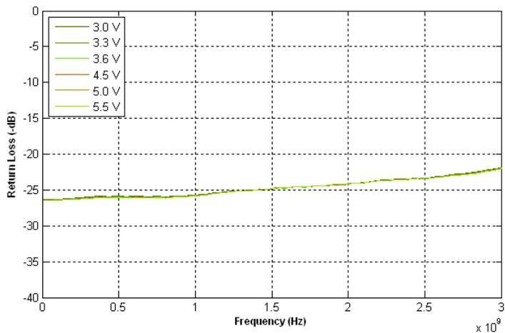
**Figure 11. Return Loss at active port @ 3.3 V**
