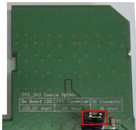
**Figure 3. Supply 3V3 from SD Connect (J6 short)**
