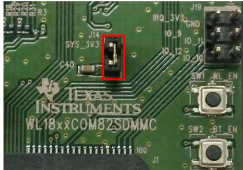
Figure 4. Supply 3V3 From FPC Connect (J14 Short)
