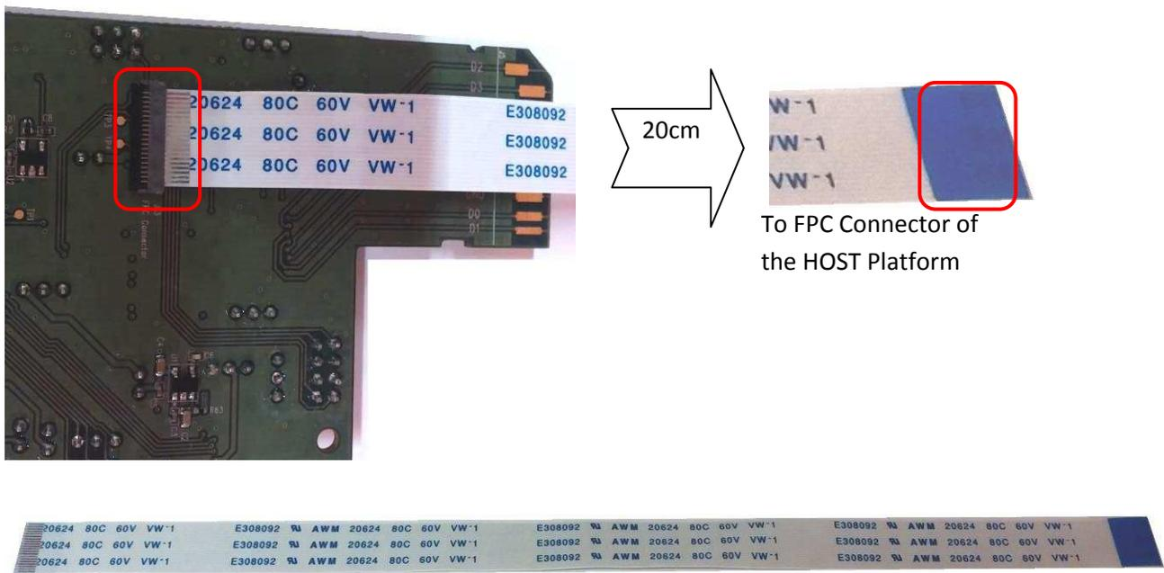
Figure 9. Connect to Platform With FPC Cable
