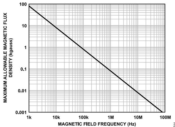
Figure 14. Maximum Allowable External Magnetic Flux Density
