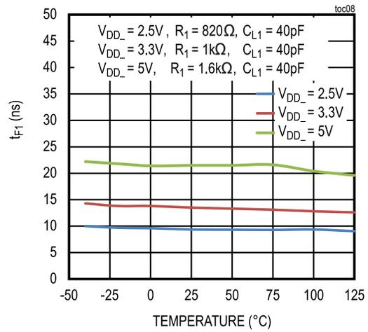
$t_{F1}$  MEASURED FROM  $0.7V_{DD1}$  TO  $0.3V_{DD1}$
