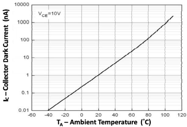
Fig 9 Collector Dark Current vs Ambient Temperature
