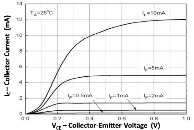
Fig 2 Collector Current vs Collector-Emitter Voltage (2)
