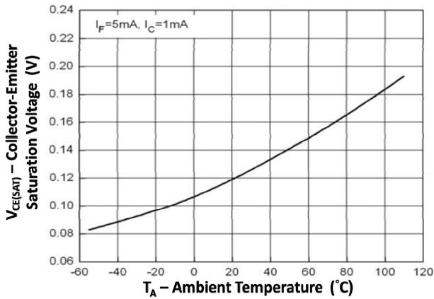
Fig 7 Collector-Emitter Saturation Voltage vs Ambient Temperature
