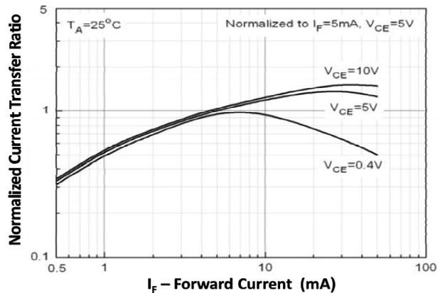
Fig 4 Normalized Current Transfer Ratio vs Forward Current
