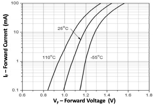
Fig 8 Forward Current vs Forward Voltage
