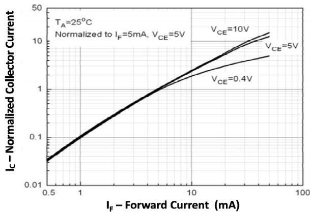
Fig 3 Normalized Collector Current vs Forward Current
