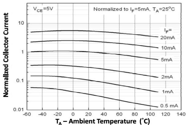
Fig 5 Normalized Collector Current vs Ambient Temperature
