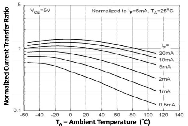
Fig 6 Normalized Current Transfer Ratio vs Ambient Temperature
