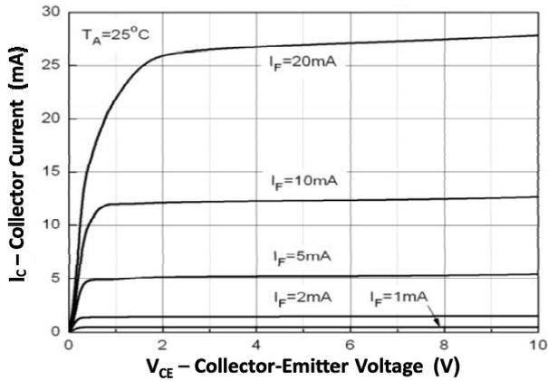
Fig 1 Collector Current vs Collector-Emitter Voltage (1)
