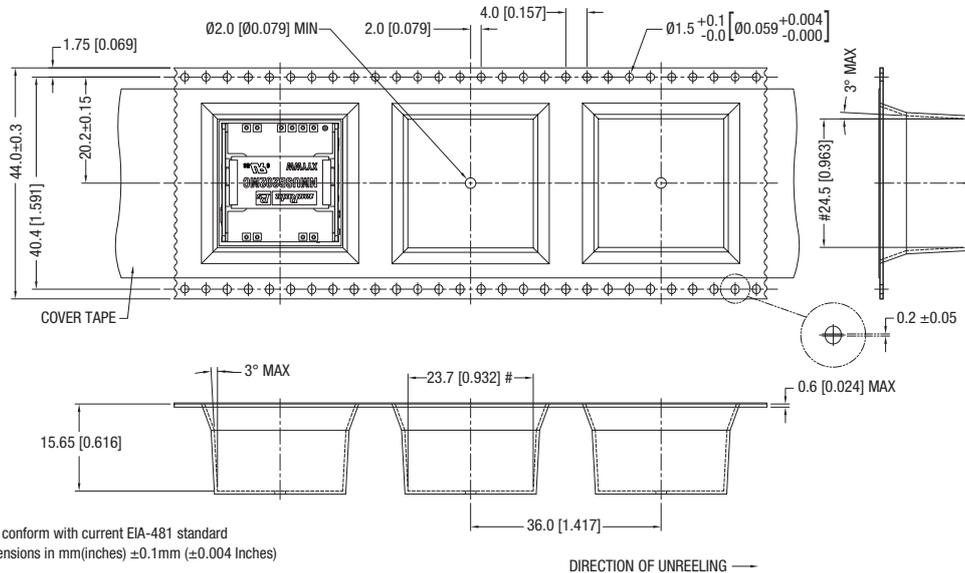
Tape & Reel specifications shall conform with current EIA-481 standard
