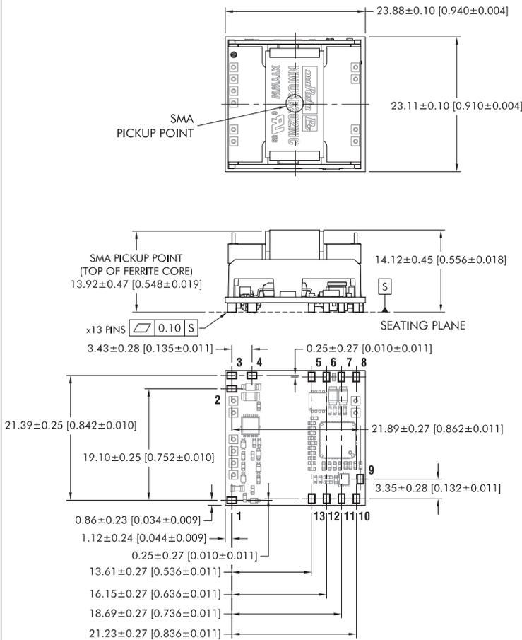
All dimensions in mm (inches), Controlling dimensions is mm.
