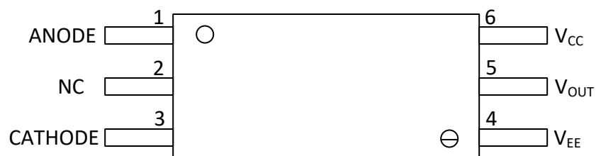
Figure 5-1. UCC23511 Package SO-6 Top View
