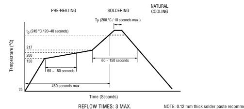
NOTE: 0.12 mm thick solder paste recommended.
