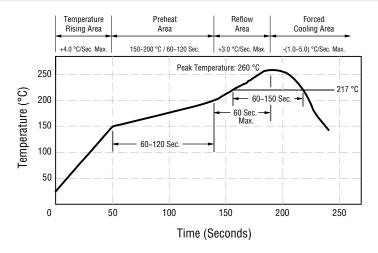
Peak Temperature: 260 °C max. Max. Peak Temperature -5 °C: 30 sec. max. Max. Time Above 217 °C: 60~150 sec. max.
