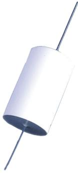
Type 935 metallized polypropylene capacitors are designed for filtering applications in switching power supplies that operate in the 20-100 kHz range. Their low ESR, high current and high capacitance gives them an advantage over general purpose types. This series is UL recognized for construction only under UL File Number E128034(N).
