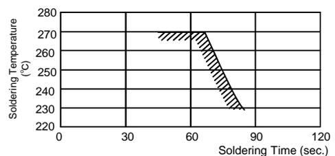
In the case of repeated soldering, the accumulated soldering time must be within the range shown above.
