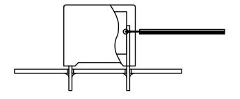
Temperature monitored inside the capacitor.
