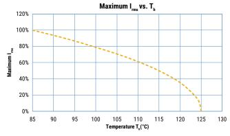
$T_h$  is the maximum ambient temperature surrounding the capacitor or hottest contact point (e.g. tracks), whichever is higher, in the worst operation conditions in °C.
