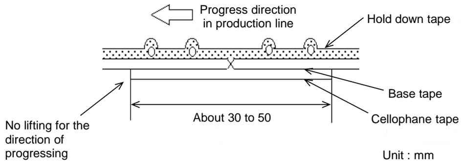
(b) When hold down tape is spliced
