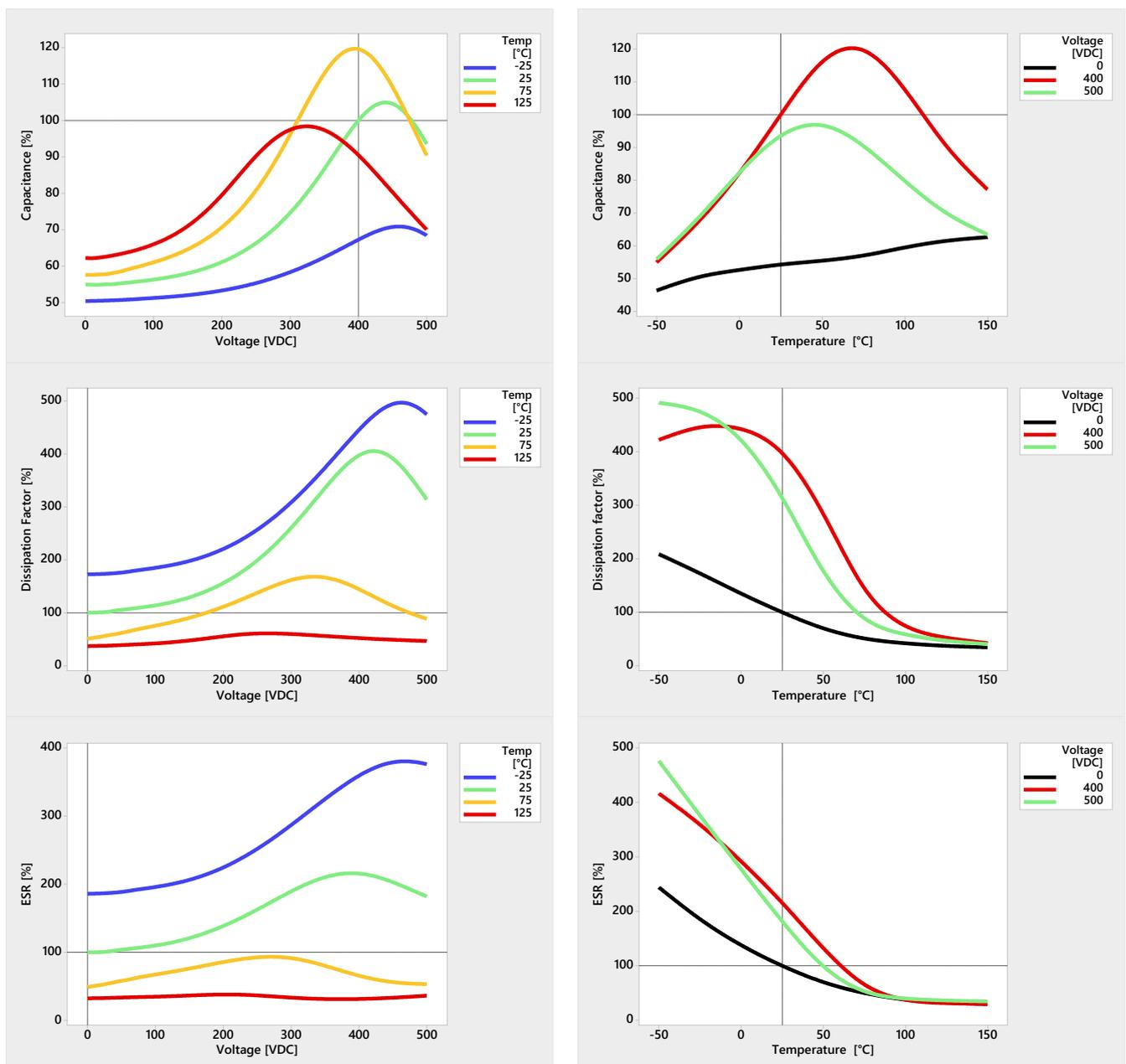
**Typical characteristics as a function of temperature and voltage -  $V_R = 900\text{ V}$**
