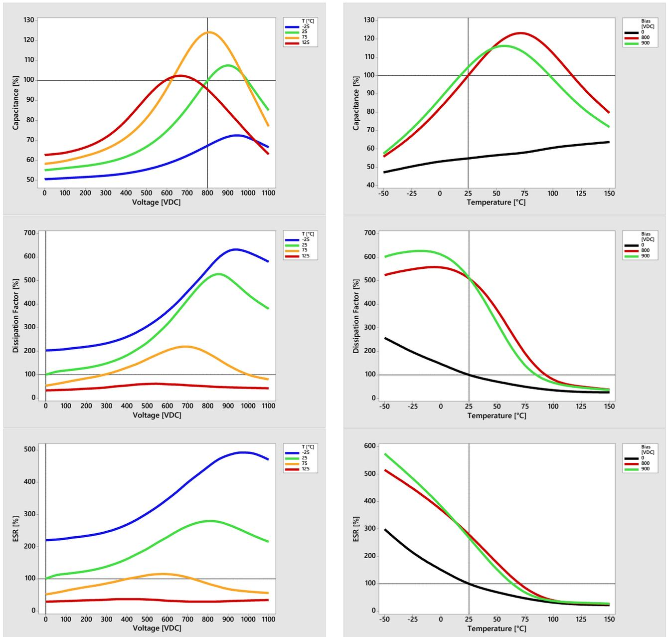
Further typical capacitance values as a function of voltage
