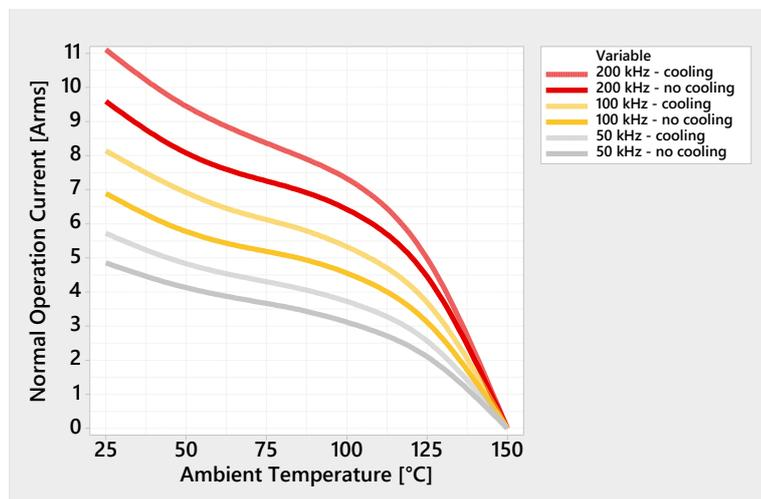
Measurement performed at  $V_{op}$ . The values correspond to a device temperature of 150 °C (measured on the ceramic surface).
