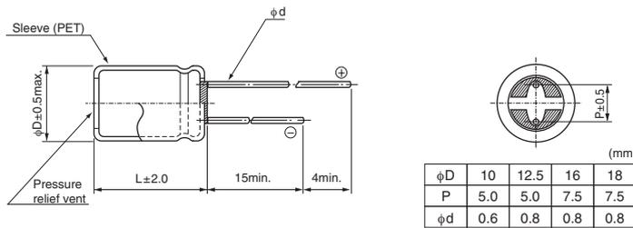
● Please refer to the Guidelines for Aluminum Electrolytic Capacitors for end seal configuration information.
