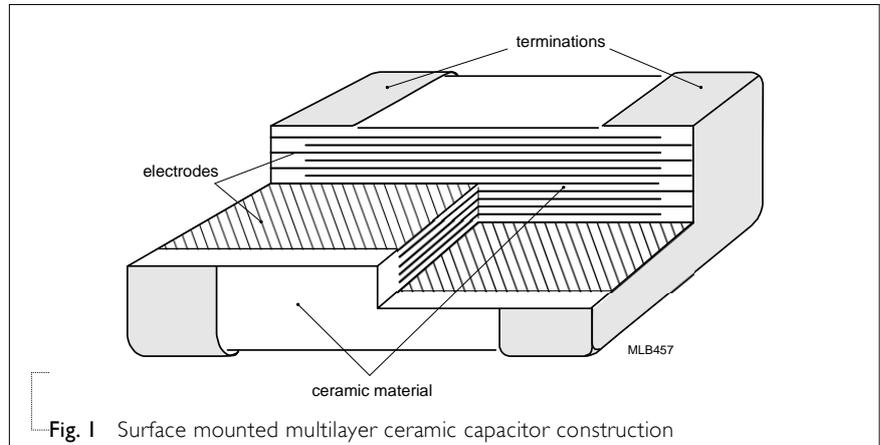
Fig. 1 Surface mounted multilayer ceramic capacitor construction
