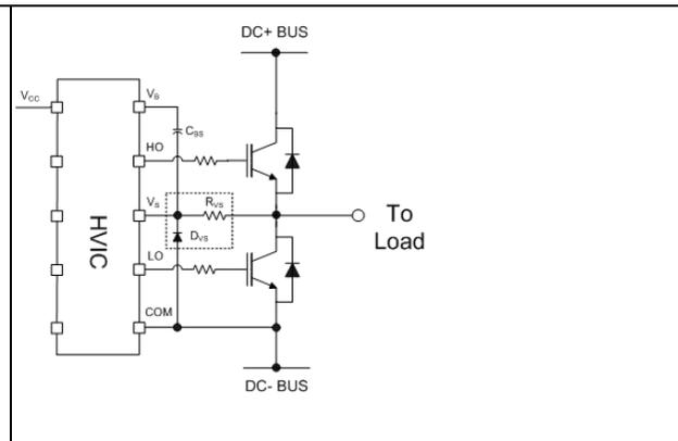
**Figure 20** Clamping diode between COM and  $V_S$
