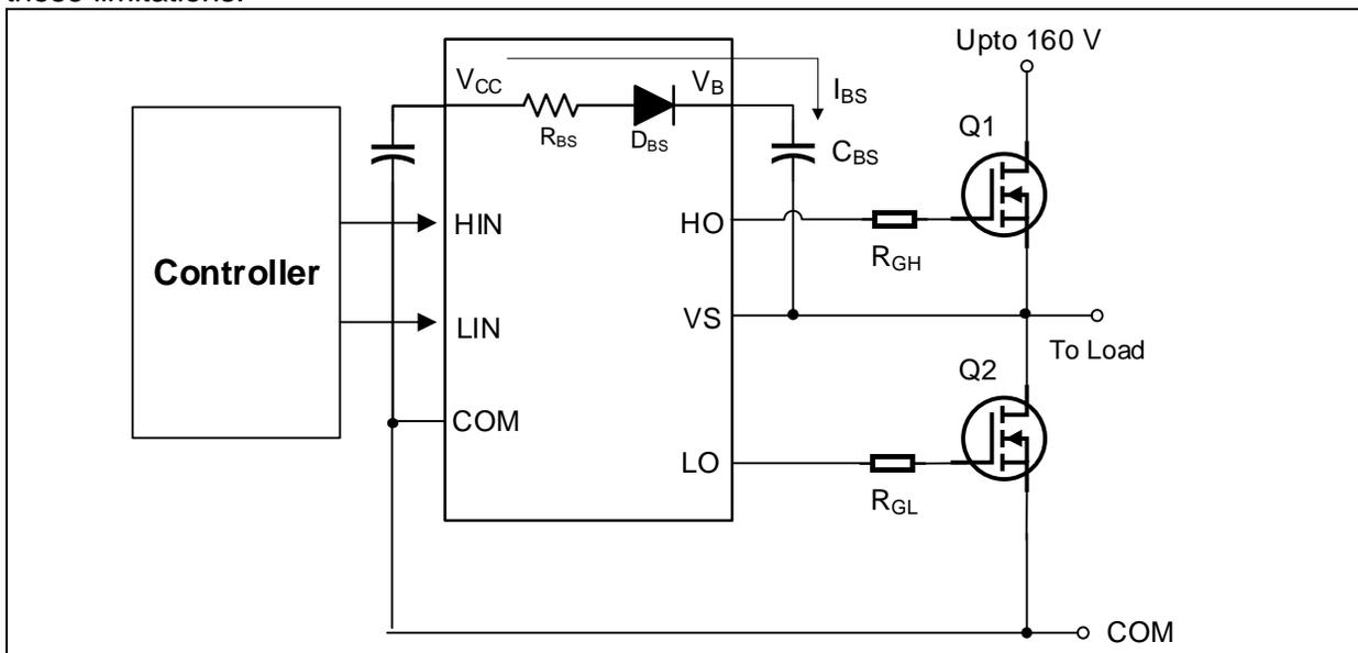
**Figure 14** Half bridge bootstrap circuit in 2ED2744S01G
