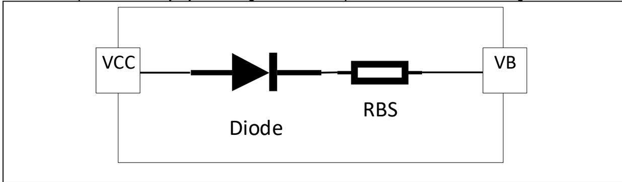
**Figure 13** 2ED2744S01G with integrated components
