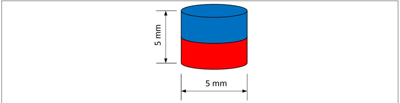
Figure 3 Magnet used in the Joystick extension
