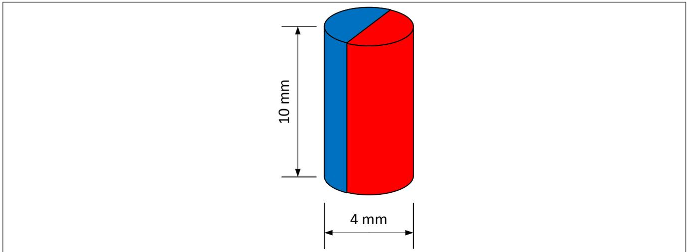
Figure 4 Magnet used in the rotation knob extension
