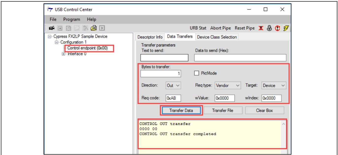
Figure 55 AA/AB Vendor Command Operation using USB Control Center
