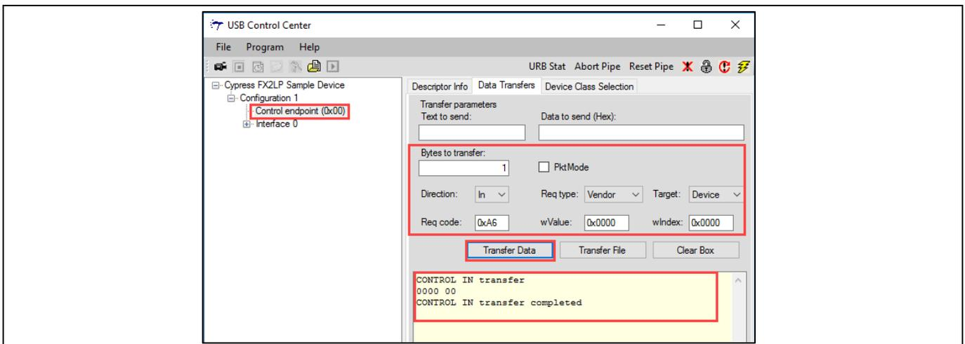
**Figure 51** A6 Vendor Command using USB Control Center
