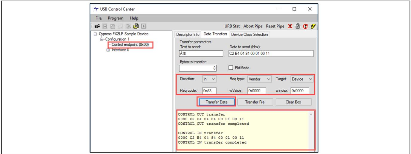
**Figure 50** A3 Vendor Command Read Operation using USB Control Center
