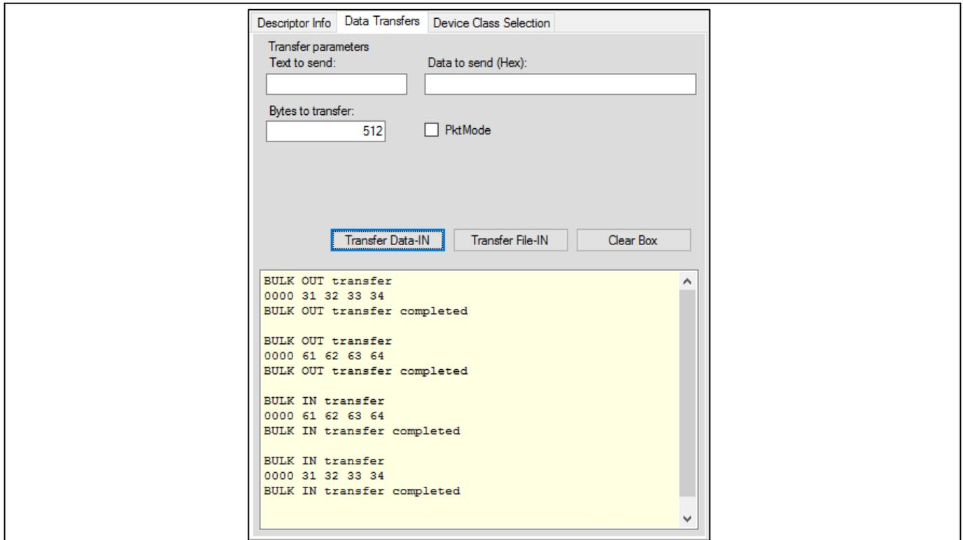
**Figure 38 Two Packets OUT, Two Packets IN**
