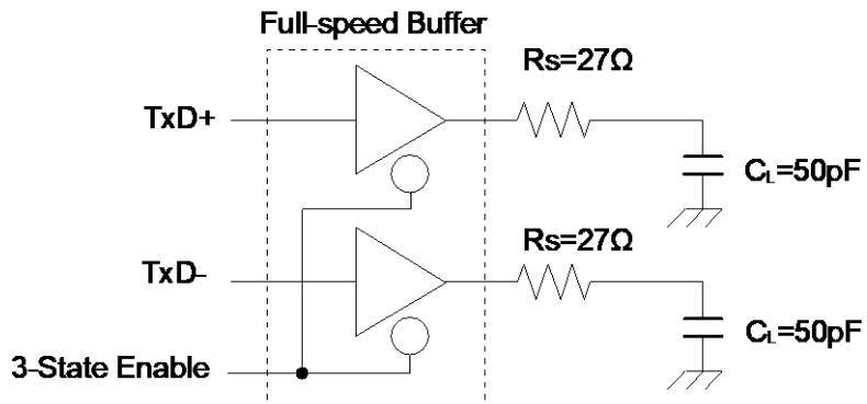
\*6: USB Full-speed connection is performed via twist pair cable shield with  $90\Omega \pm 15\%$  characteristic impedance (Differential Mode). USB standard defines that output impedance of USB driver must be in range from  $28\Omega$  to  $44\Omega$ . So, discrete series resistor ( $R_s$ ) addition is defined in order to satisfy the above definition and keep balance. When using this USB I/O, use it with  $25\Omega$  to  $30\Omega$  (recommendation value  $27\Omega$ ) series resistor  $R_s$ .
