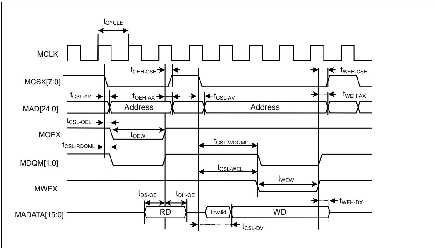
**Separate Bus Access Synchronous SRAM Mode**
