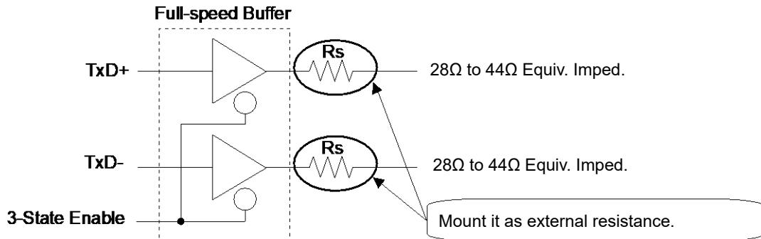
$R_s$  series resistor  $25\Omega$  to  $30\Omega$
