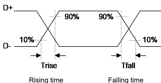
See Figure "Low-Speed Load (Compliance Load)" for conditions of external load.
