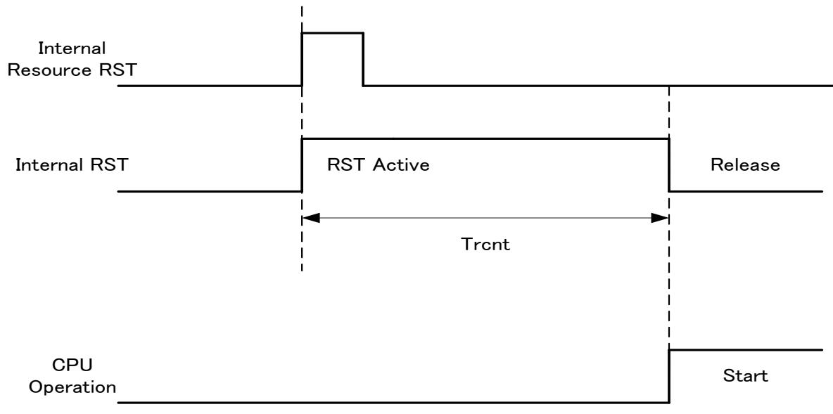
\*: Internal resource reset is not included in return factor by the kind of Low-Power consumption mode.
