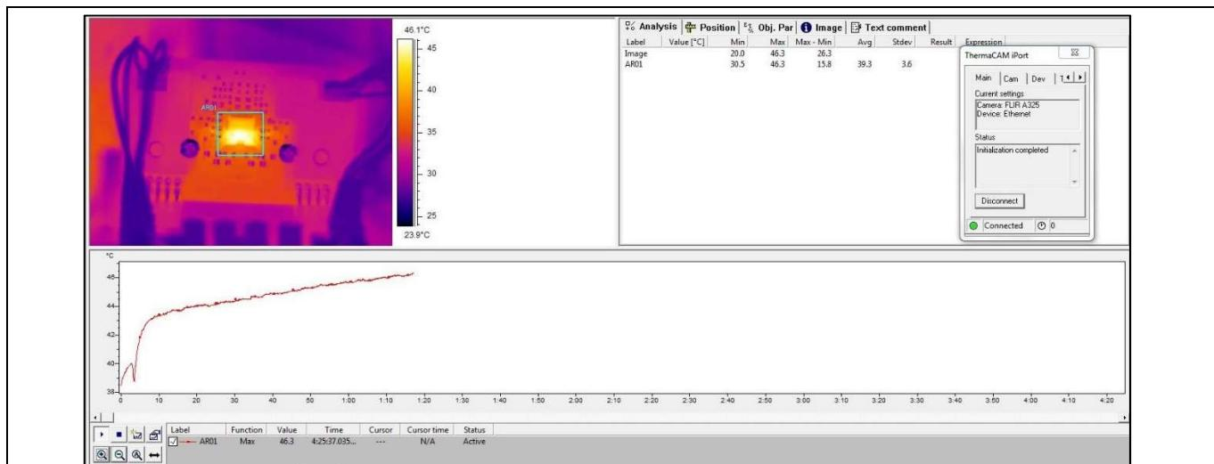
**Figure 9 Peak power  $P_{out} = 103 \text{ W}$  with  $6 \Omega$  load  $\pm 32 \text{ V}$**
