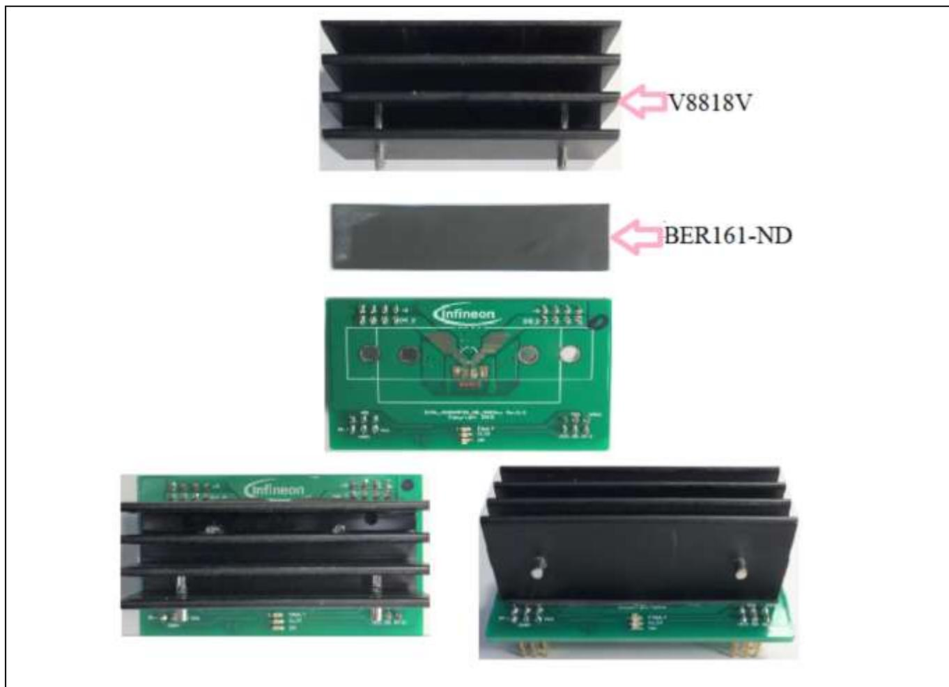
**Figure 15     Heatsink installation**
