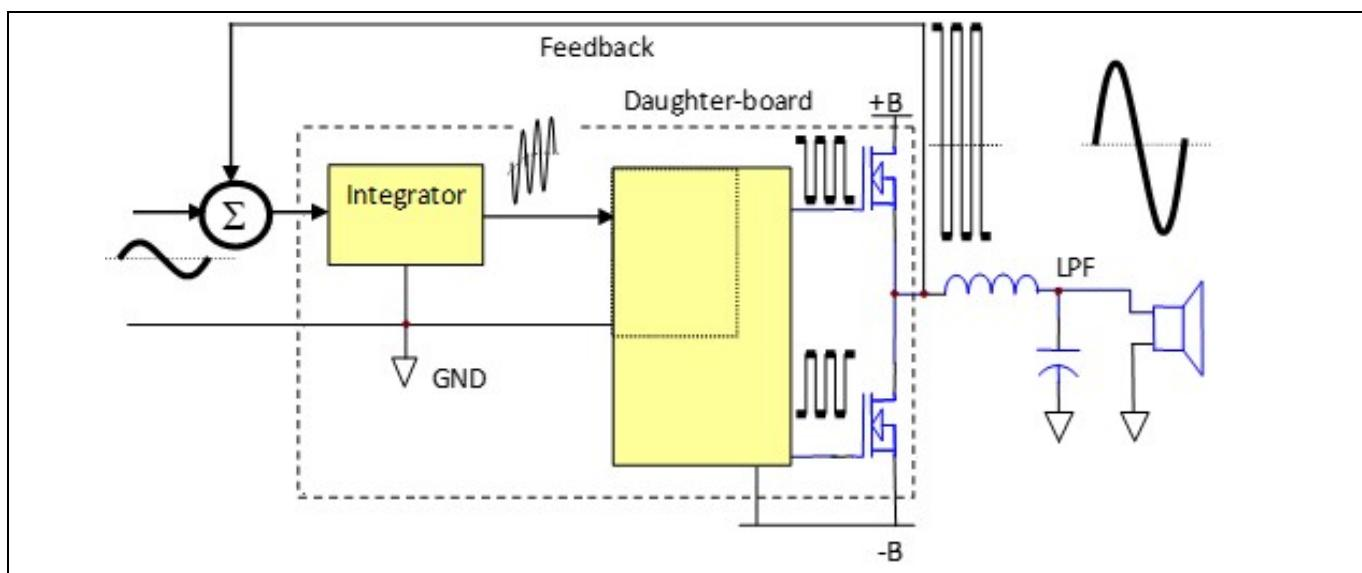
**Figure 1** Simplified block diagram of class D amplifier
