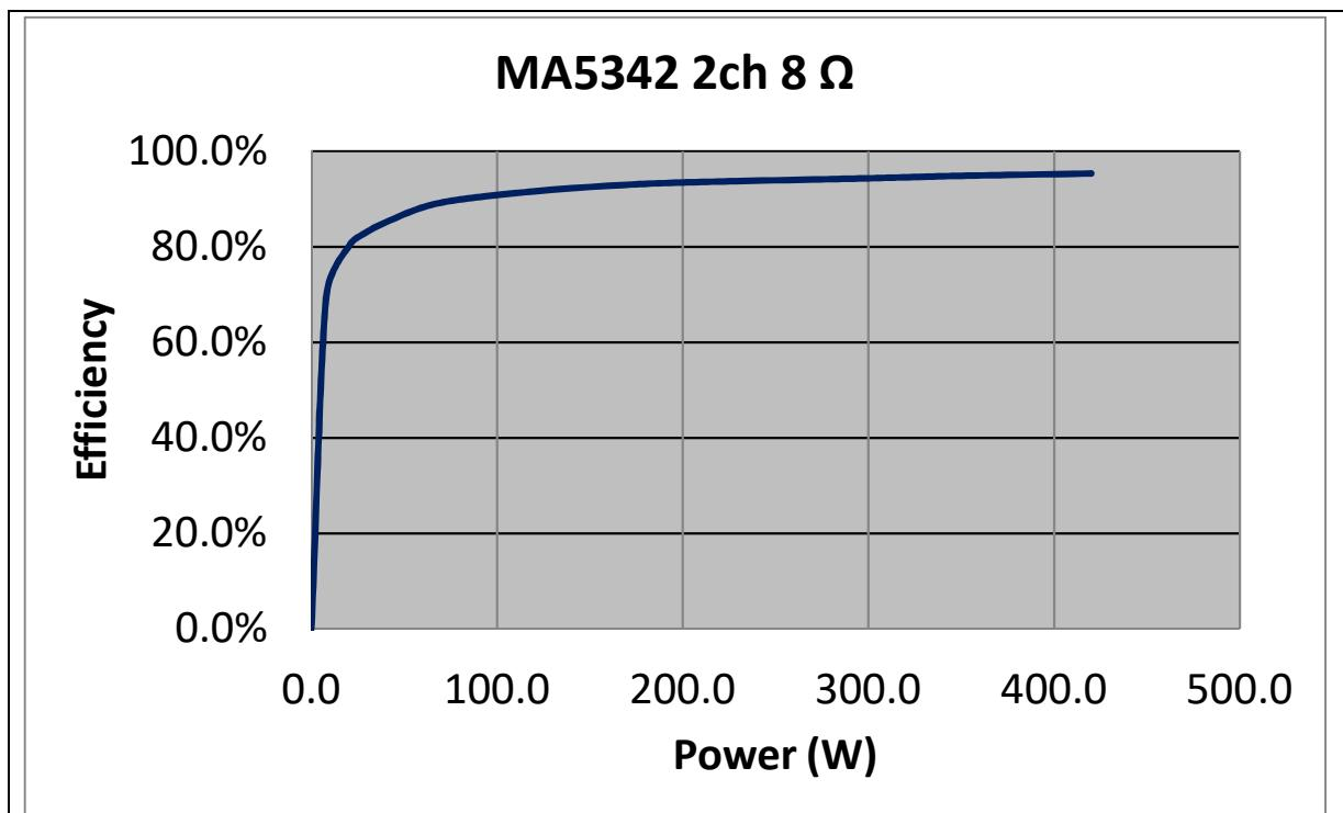
Figure 8 EVAL\_MA5302MS\_200X2 8 Ω load stereo, ±B supply = ±52.2 V
