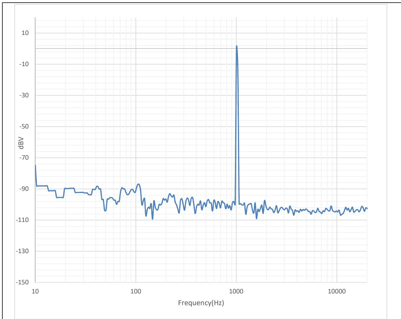
**Figure 7**      **Noise floor with 1 V<sub>RMS</sub> output 8 Ω load**
