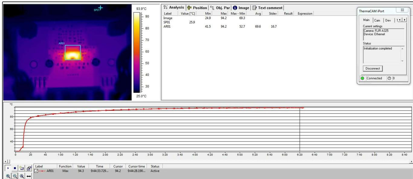
**Figure 9 Peak power  $P_{out} = 210$  W with  $8 \Omega$  load  $\pm 52.2$  V**
