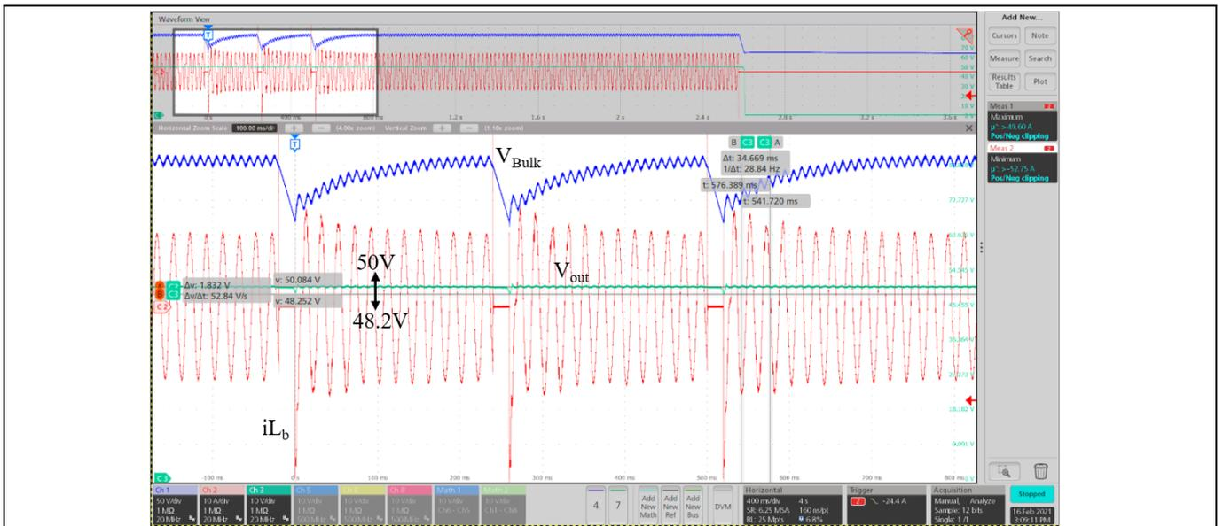
**Figure 37** Detail view of 20 ms hold-up time at 60 A load and 230 V<sub>AC</sub>
