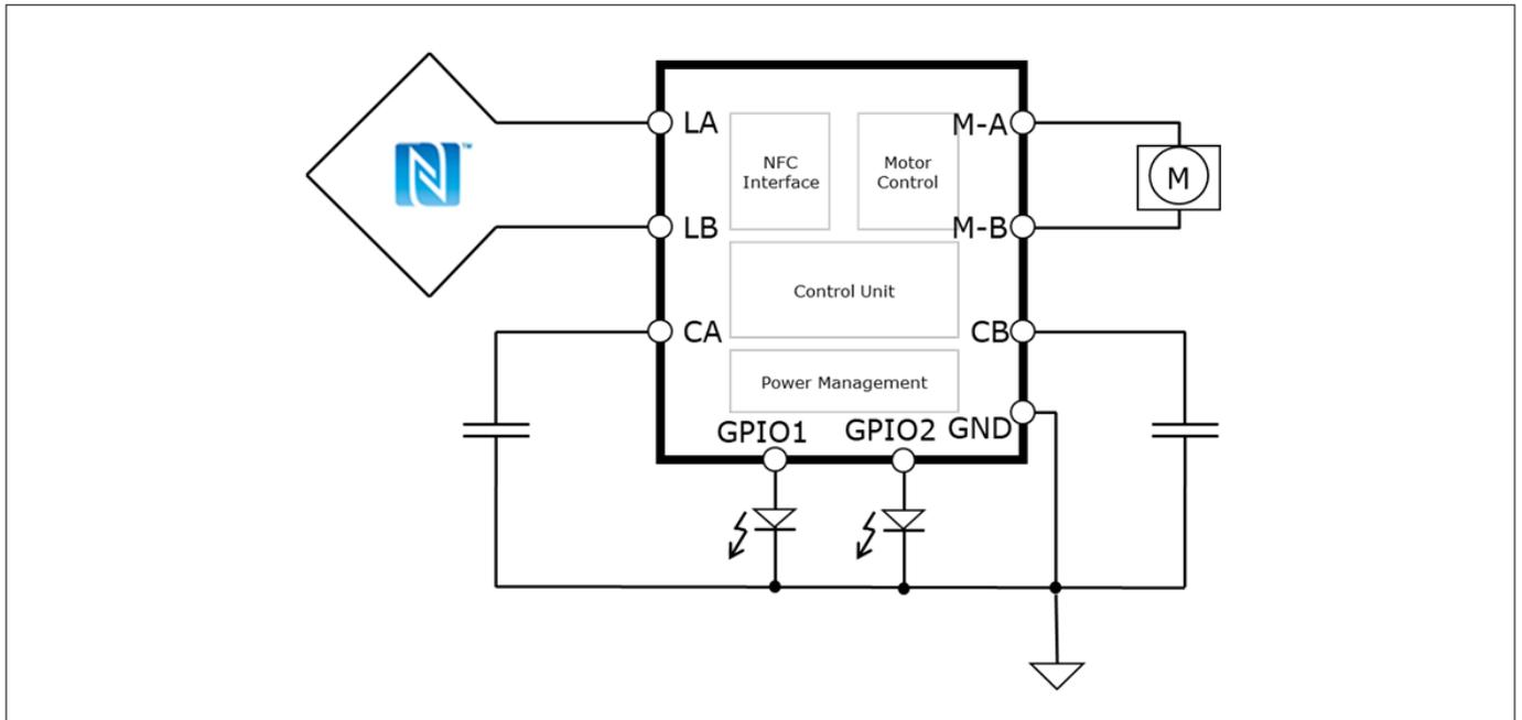
Figure 1 Smart Lock Example (Passive Supply Mode )
