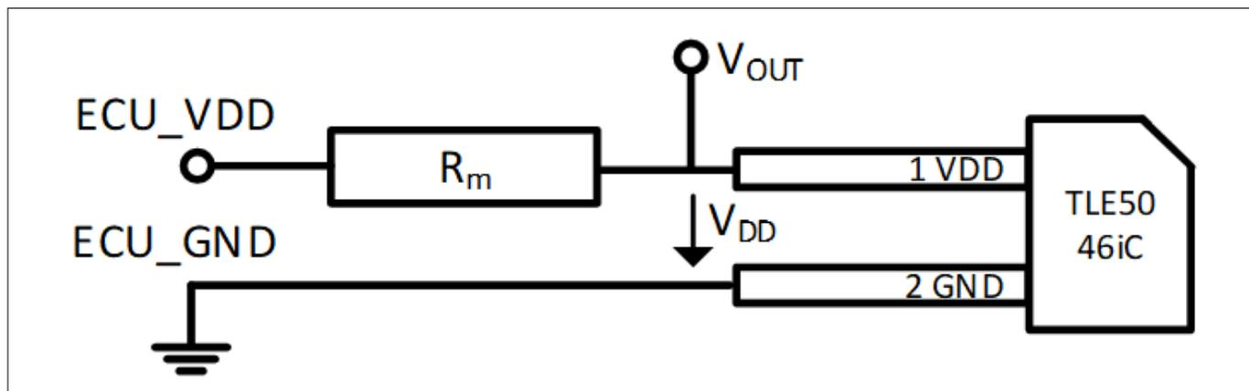
Figure 5 Pin configuration
