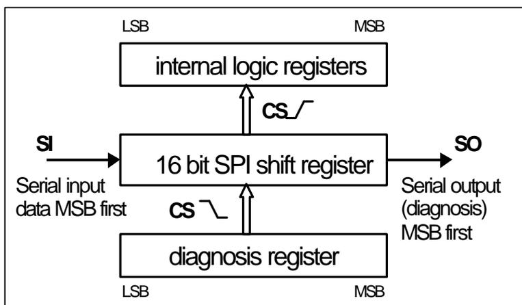
**CS = H:** Any signals at the SCLK and SI pins are ignored and SO is forced into a high impedance state.
