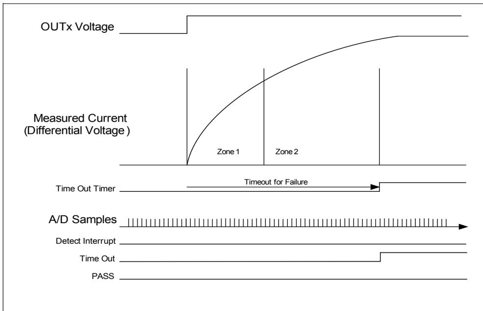
Figure 17 Current Profile Diagram - Time Out Failure
