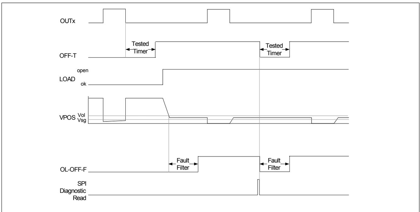
Figure 13 Off-State Diagnostics Timing Diagram - open
