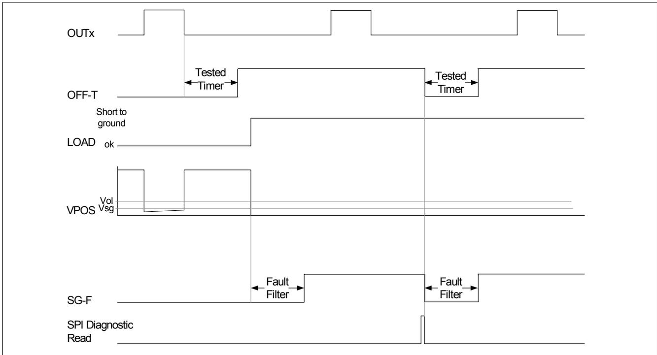
Figure 14 Off-State Diagnostics Timing Diagram - short to ground
