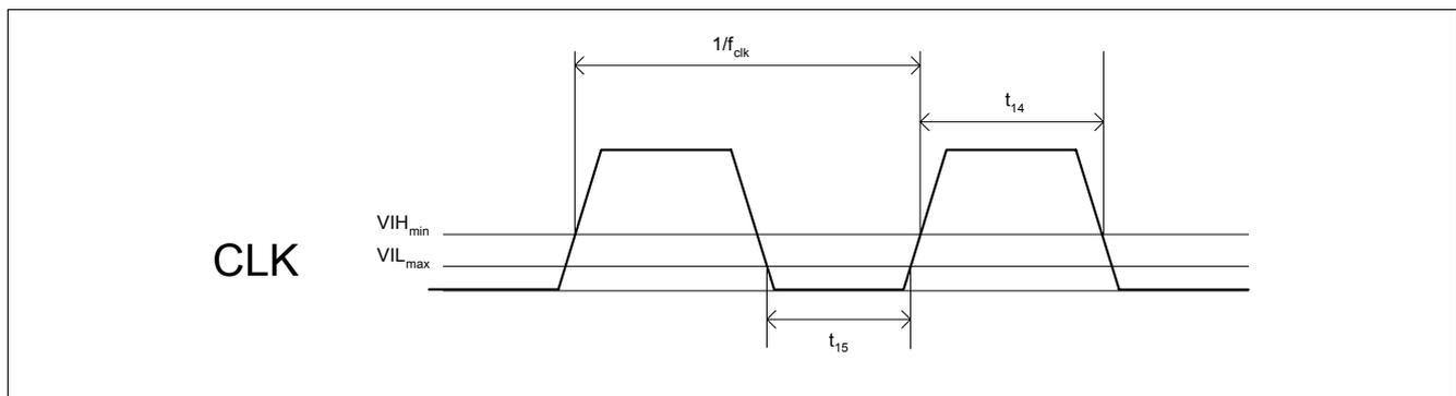
Figure 7 CLK Timing Diagram
