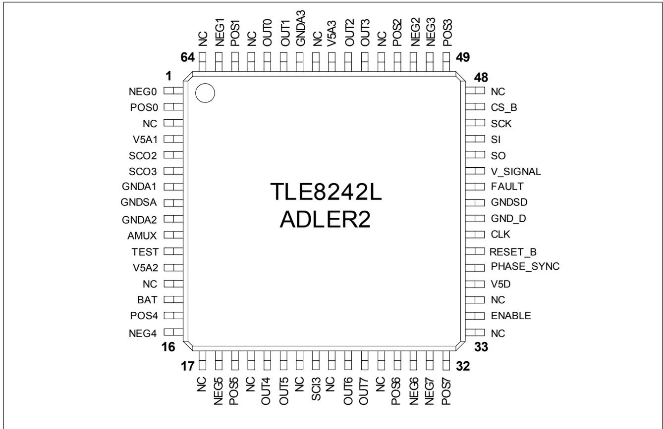
Figure 6 Pin Configuration
