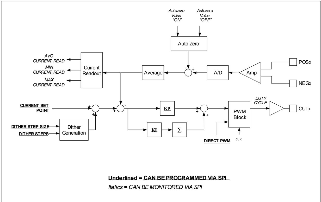
**Figure 3 Control Loop - Simplified Diagram**
