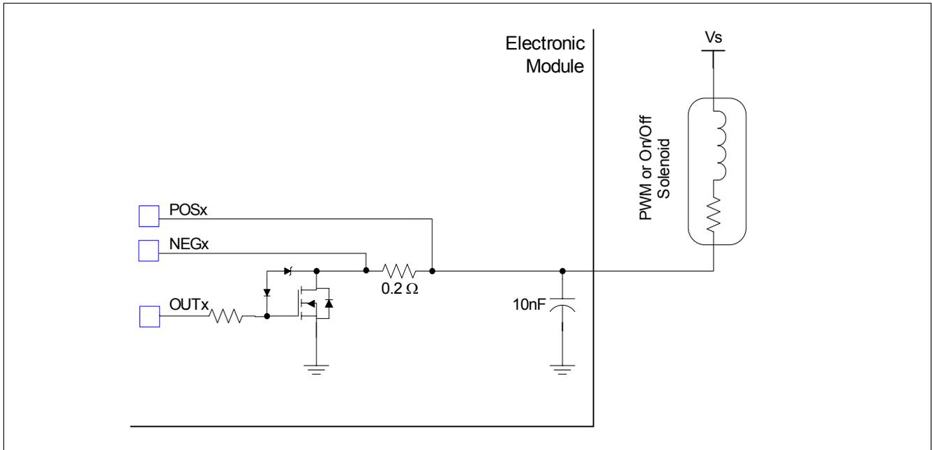
Figure 1 External Circuit Diagram for Direct PWM Mode Operation
