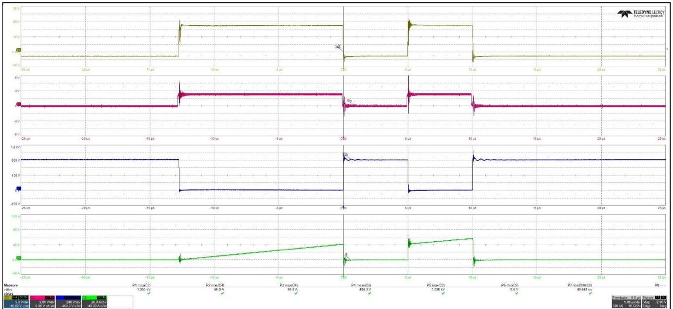
**Figure 4 Eval-1ED3142MU12F-SiC – Double-pulse test of the low side CoolSiC™ MOSFET with 18V / -3V bipolar power supply**
