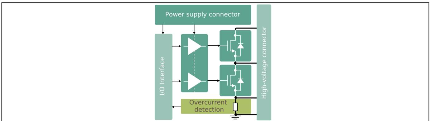
**Figure 2 Eval-1ED3142MU12F-SiC evaluation board block diagram**
