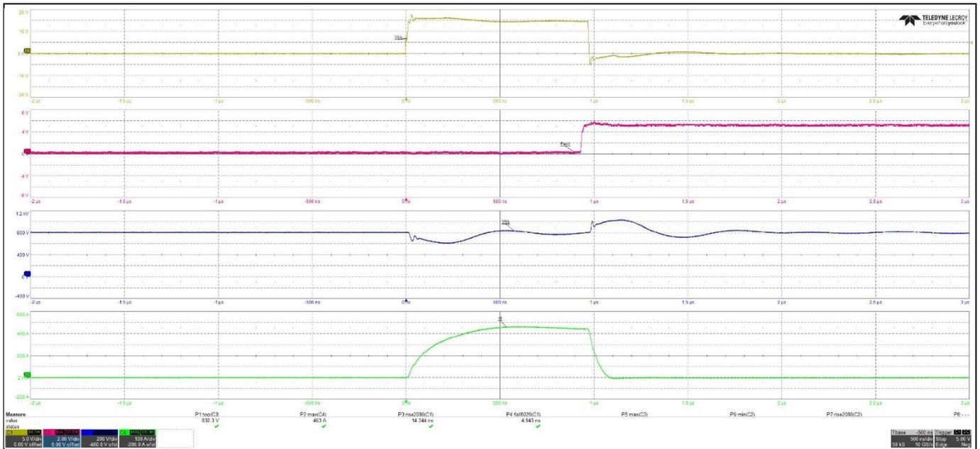
Figure 5 Eval-1ED3142MU12F-SiC – Overcurrent protection in case of short-circuit
