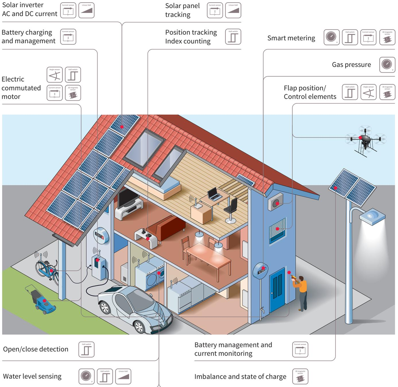
Our broad and deep sensor offering provides the perfect fit for various industrial/home applications, including renewable energy, white goods, home automation, drones and power tools. In the home appliances sector, electric commutated BLDC drives are being increasingly used to reduce
