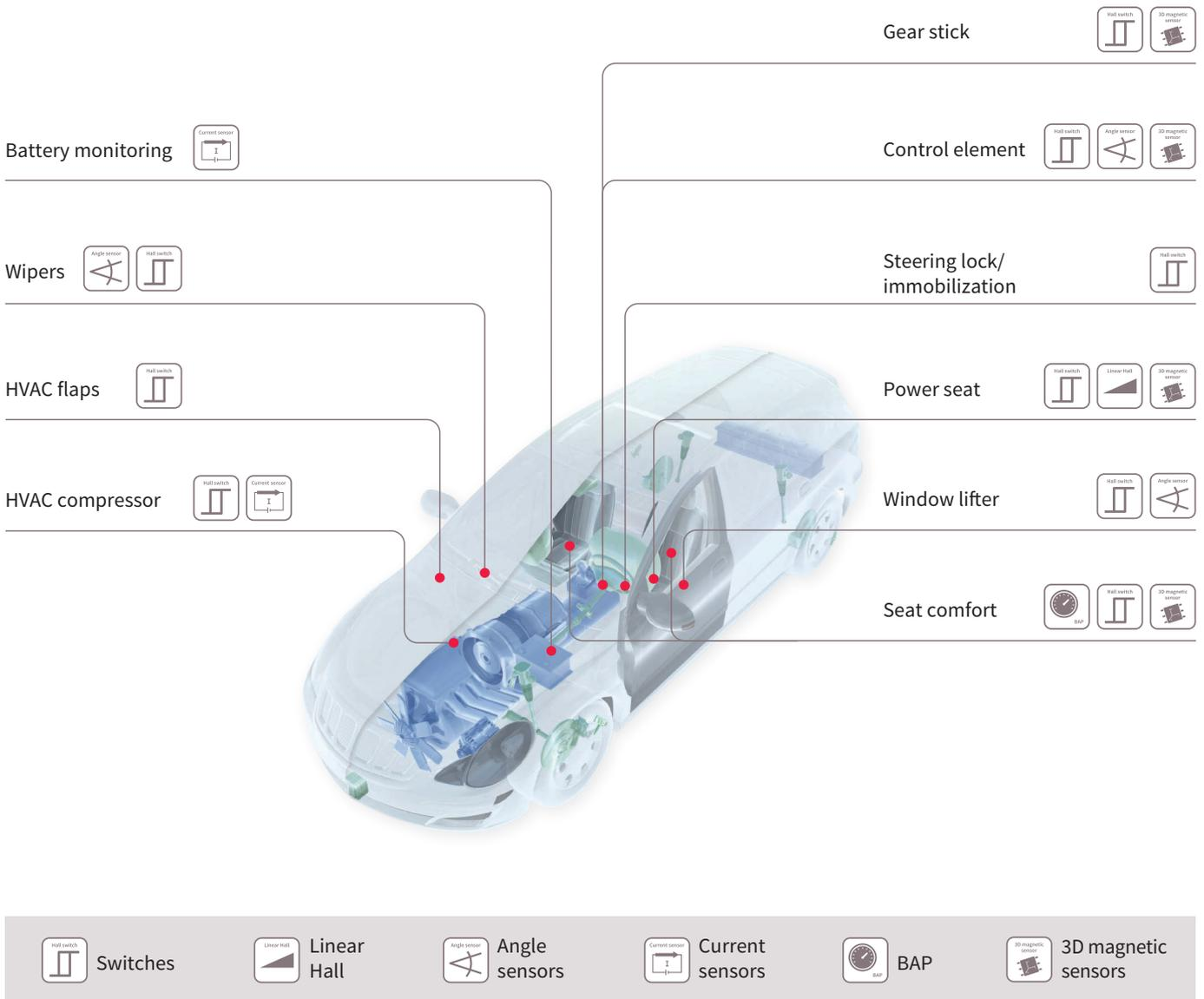
The body segment presents the most diverse target market for sensors. Hall switches, for example, are deployed in classic applications such as window lift modules, whereas
