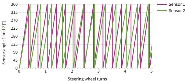
The angle sensors for absolute steering angle measurement are available as a single-sensor SMD package for conventional designs, which achieve the ASIL-D rating via a plausibility calculation of the two angle sensor signals
