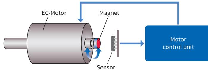
A correct commutation of the EPS motor has to be ensured, in order to avoid a blocked steering or the erratic steering support. This application is also classified in the category of ASIL-D. To achieve this high level of functional safety, Infineon offers angle sensors in the dual-sensor package that allow the integration of two redundant sensors in the place of one.
