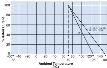
For resistors operated at an ambient temperature of 70°C or above, a current rating shall be derated in accordance with the above derating curve.
