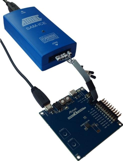
Figure 7-2. SAM-ICE using an Atmel-ICE Adapter
