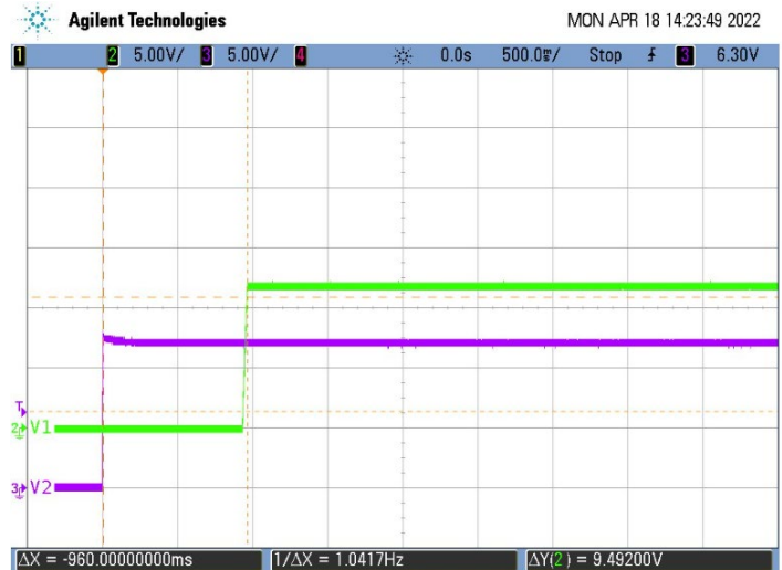
Figure 4: V1 V2 Power-on-Delay
