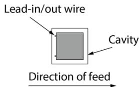
\* The packing direction of the chip coils in the taping is unified with the in/out positions of the lead wires.
