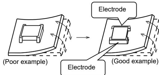
(2) Components location on PCB separation
