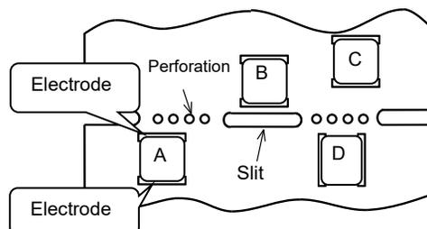
**(3) Mounting components near screw holes**
