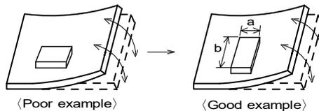
(2) Components location on PCB separation
