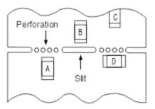
(3) Mounting components near screw holes
