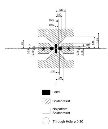
$<sup>^{\</sup>star}$  Line width to be designed to match  $50\Omega$  characteristic impedance, depending on PCB material and thickness.
