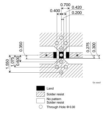
\* Line width to be designed to match 50 ohm characteristic impedance, Depending on PCB material and thickness.
